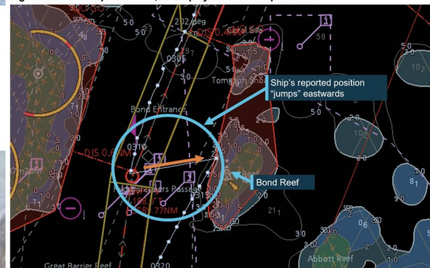
Figure 5: Rosco Poplar's track, as displayed on the ship's ECDIS
